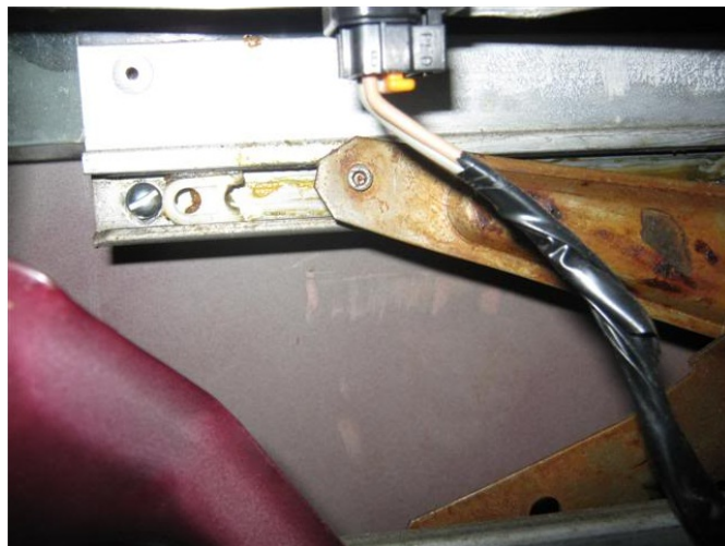
Crimped end and broken roller.
