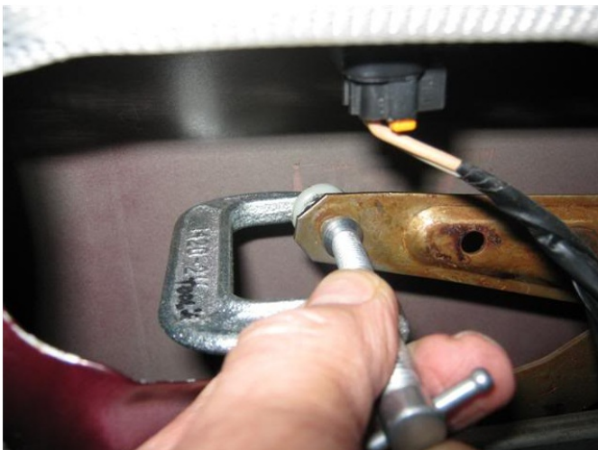
Pressing in the ball stud into the new roller.
