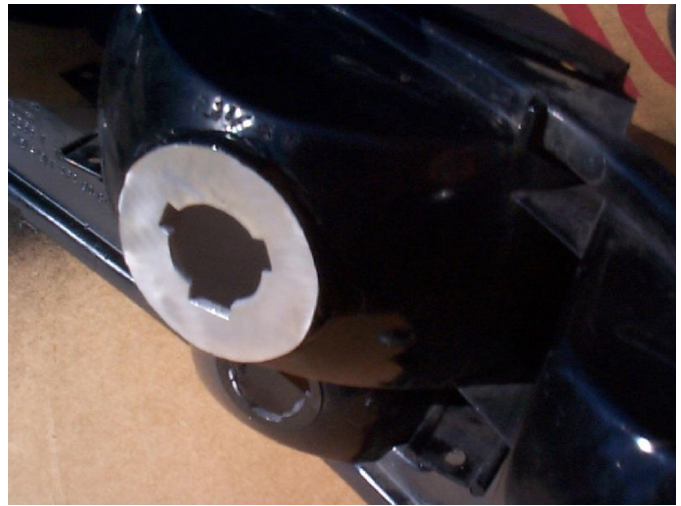
Locking ring glued in place.
